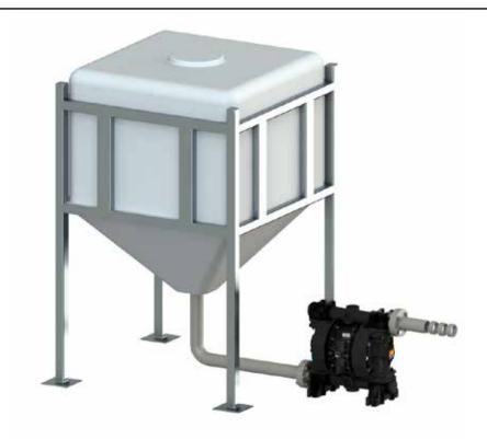
Pump installed on hopper for high viscosity liquid (hopper's height helps the pump to treat the fluid. Air pressure has to be high, suction tube has to be bigger than pump size)
